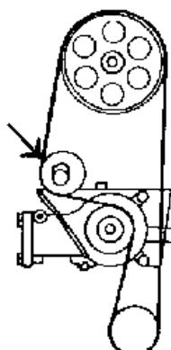
When you change the water pump, it is recommendable to check the belt and the adjustable gear, and replace them if they are worn.
