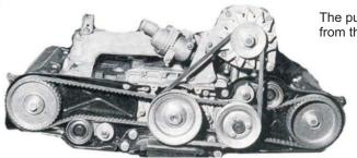
The pump is driven by a timing belt, which is shared with the alternator from the crankshaft.
